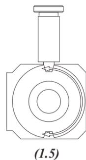
5. Move forward the grinding wheel and grind the cutting lips, after keeping the attachment horizontally.
