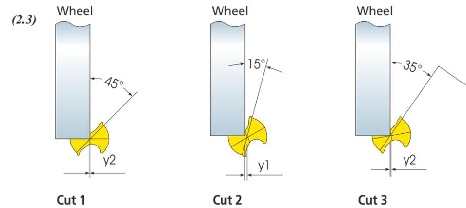
4. Grind as procedure <cut 1>,<cut 2>, <cut3>.(see 2.3)
