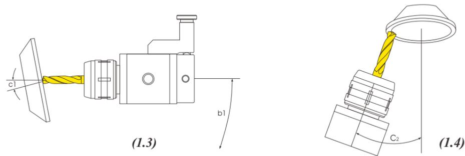
3. Set the cutting edge toward grinding wheel to the point angle <c1, 8°> as shown (1.3). Then, keep the angle <c2, 20°> as shown (1.4).
