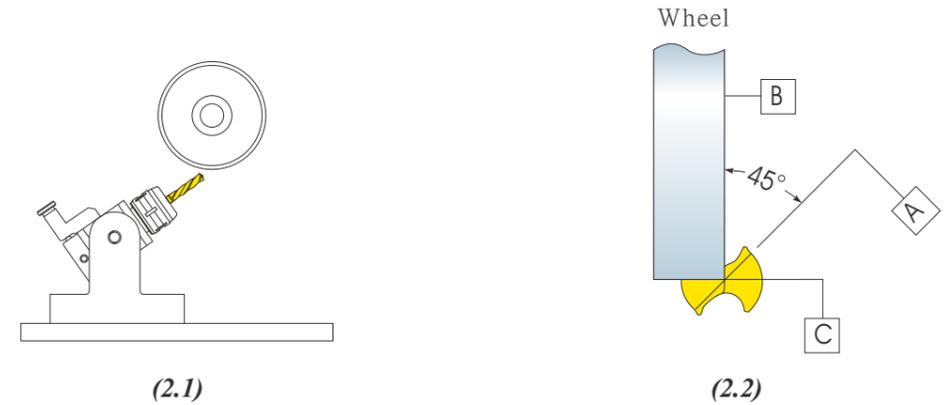
1. Set the drill at 30° or 35° in the drill attachment.(see 2.1) (In case of drill for AL, FC material, keep 30°, while others at 35°.)
