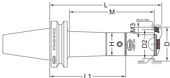
**整支 SET****MAS403 BT-HBIT 粗搪孔刀－反搪-AK type****MAS403 BT and HBIT Adjustable Single Reverse Cutter Boring Head**
