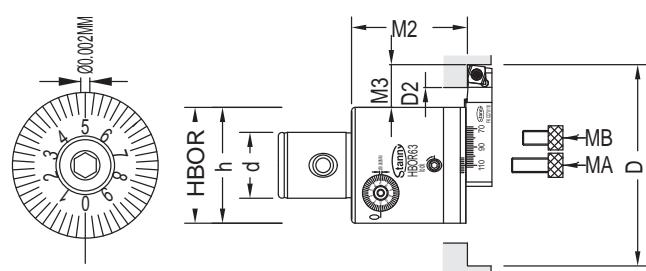
**HBOR 極細微調精搪孔刀－菱形反搪****HBOR Micro-Finishing Cutter for Rhombus Reverse Fine Boring Head**
