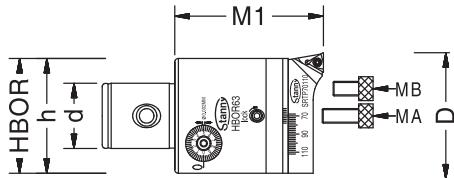
**HBOR 極細微調精搪孔刀****HBOR Micro-Finishing Cutter Fine Boring Head**
