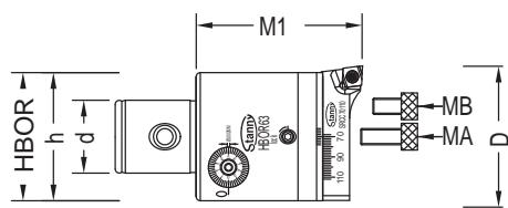
**HBOR 極細微調精搪孔刀 – 菱形****HBOR Micro-Finishing Cutter for Rhombus Fine Boring Head**
