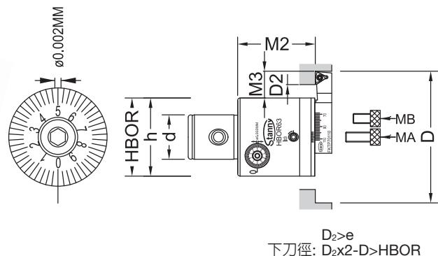
**HBOR 極細微調精搪孔刀－反搪****HBOR Micro-Finishing Cutter for Reverse Fine Boring Head**
